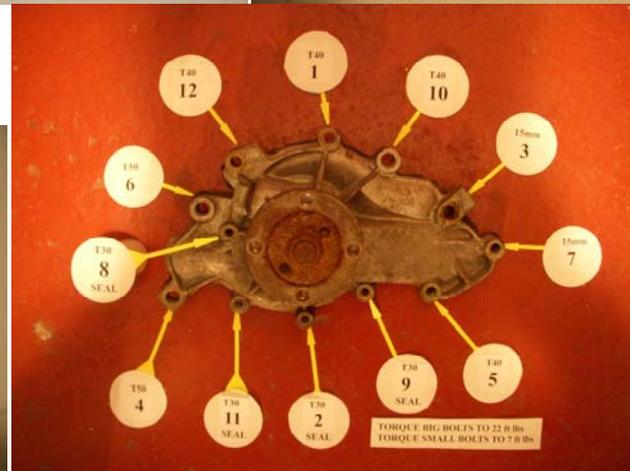
The water pump on a Fiero works hard to circulate coolant around the whole car. It lives in a hostile area filled with hot chemicals but soldiers on for years. Eventually though you begin to hear a low pitch rumble or you see a little green drip by the right rear tire. Soon you must get to know the water pump up close and personal.
